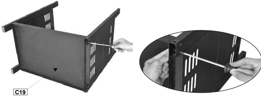
Attach the left / right cabinet panel assembly to the Bottom Panel (C19) using M6x40 Bolts (D5x8pcs) and M6 Nuts (D6x8pcs) as shown.
