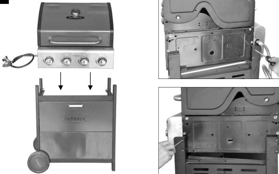
Carefully place the Barbecue Body (B1) onto the cabinet structure and fix using M6x40 Bolts (D5x8pcs) as shown.
