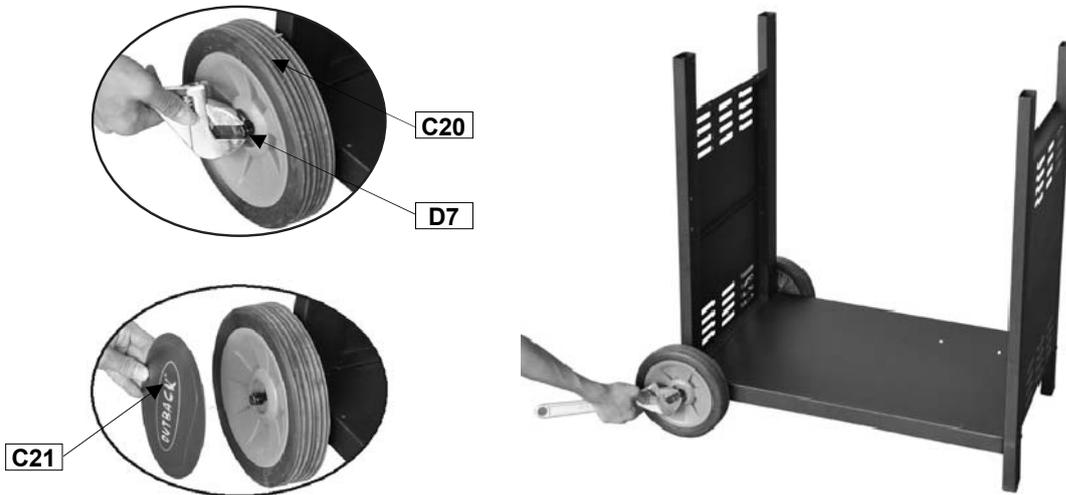
Unscrew the Locknuts (D7) from both ends of the Axle (C22).
