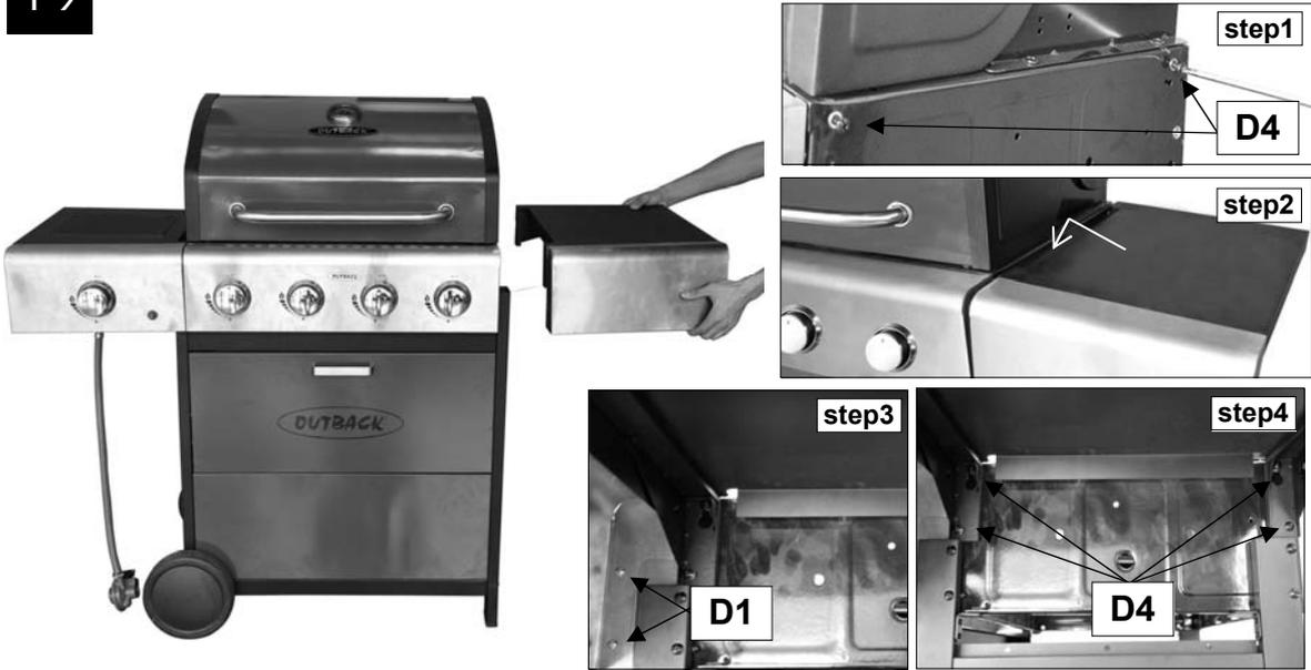
Attach the side shelf assembly to the barbecue body using ST4.0x10 Screw (D1x2pcs) and M6x15 Bolts (D4x4pcs) as shown.
