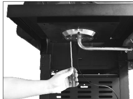
Feed the venturi tube of the Side Burner (C7) through the hole in bottom of the side burner shelf, and fix it onto side burner shelf using a M4x10 Bolt (D2) as shown. Make sure that the end of venturi tube is set over the gas outlet of side burner valve.
