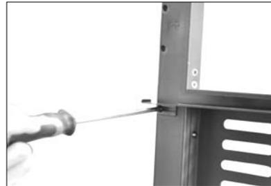
Attach Drip Tray Left Bracket (B8) to the left legs using ST4.0x10 Screws (D1x2pcs) as shown. Repeat above process for Drip Tray Right Bracket (B9).
