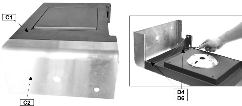
Attach Side Burner Shelf Panel (C2) onto Side Burner Shelf (C1) using M6x15 Bolts (D4x2pcs) and M6 Nuts (D6x2pcs).
