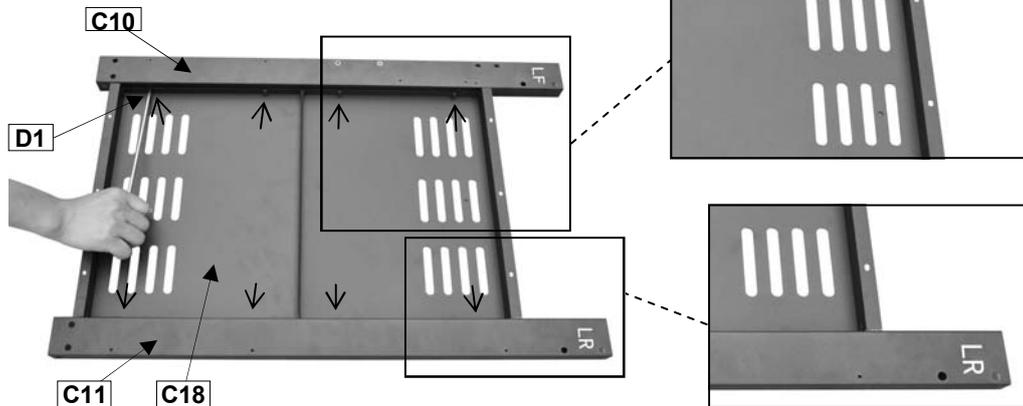
Attach the Left Legs (C10,C11) to the Side Panels (C18x2pcs) using ST4.0x10 Screws (D1x8pcs) as shown.
