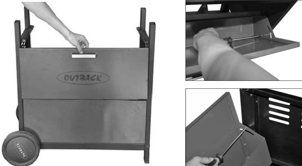
Install the storage box assembly between left / right front legs using M4x10 Step Bolts (D3x4pcs).
