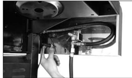
Unscrew the pre-assembled nut of the Ignition Button (C6).
