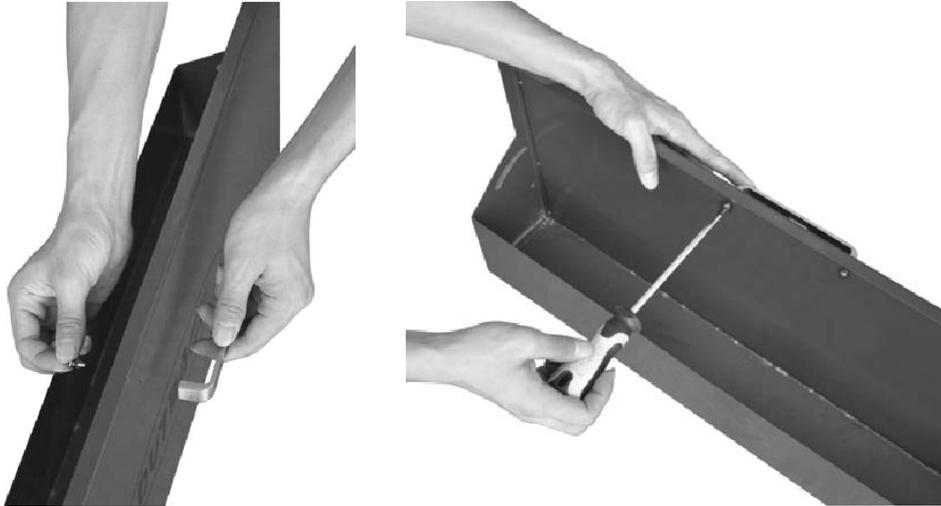
Remove the retaining bolts from Storage Box Handle (C15), then fix it onto Storage Box (C16) using the retaining bolts.
