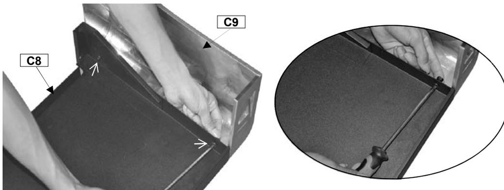
Attach Side Shelf Panel (C9) onto Side Shelf (C8) using M6x15 Bolts (D4x2pcs) and M6 Nuts (D6x2pcs).
