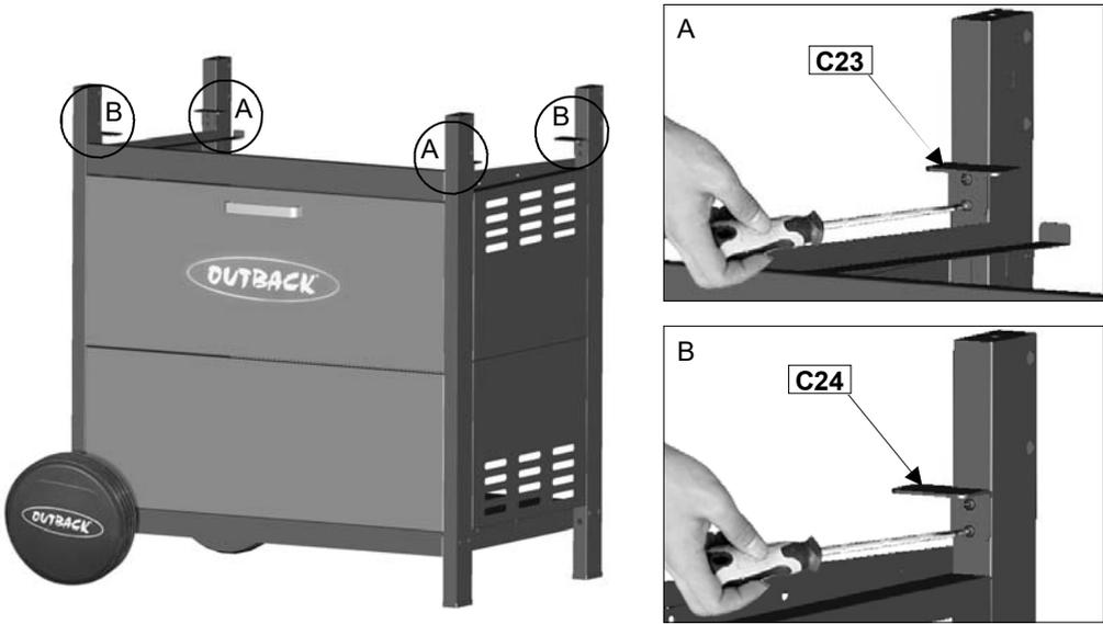
Remove the retaining bolts from legs, then attach Body Support A (C23) onto the left rear leg and right front leg, and attach Body Support B (C24) onto the right rear leg and left front leg using the retaining bolts.
