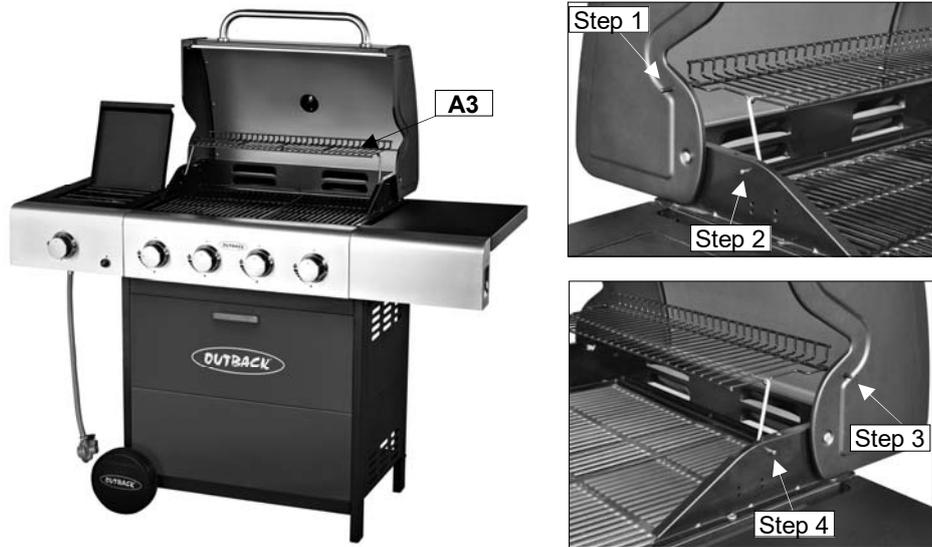
Attach the Warming Rack (A3) to the hood and barbecue body as shown. Make sure that the swing legs fix to the body of the barbecue and the shorter fixed legs go through the holes in the hood.
